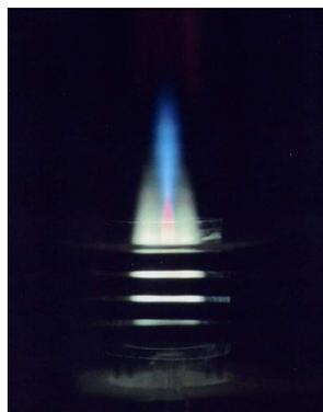
Samples are analysed by ICP-AES
