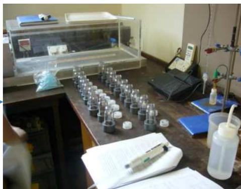
Soil samples are weighed into centrifuge tubes
